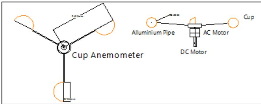
Figure 2: Cup anemometer and DC motor.
