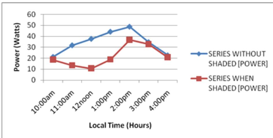
Figure 4: Graph of Power output at various time for series connection
