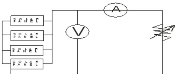
Figure 2: Parallel Connection of Solar Panel
