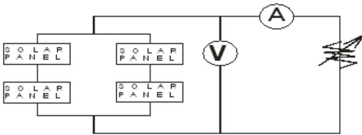
Figure 3: Series-Parallel connection of solar panel
