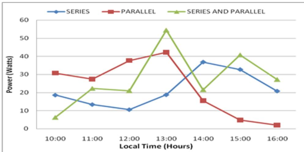
**Figure 7:Comparism of shaded PV power output at various times for Series, Parallel and Series/Parallel connections**
