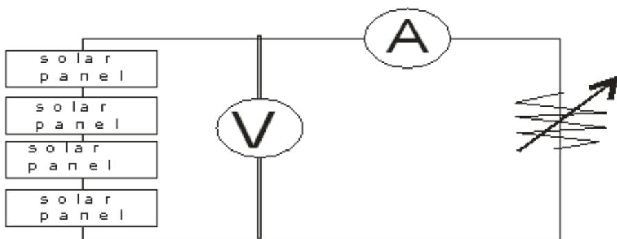
Figure 1: Series Connection of Solar Panel
