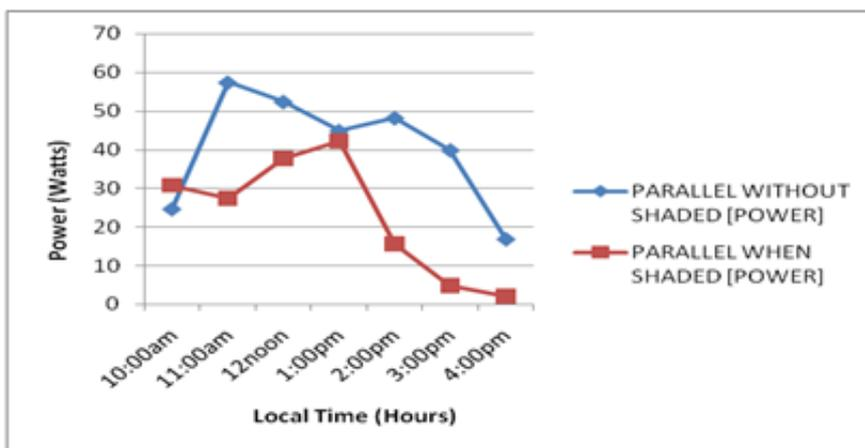
Figure 5: Graph of Power against time in parallel connection
